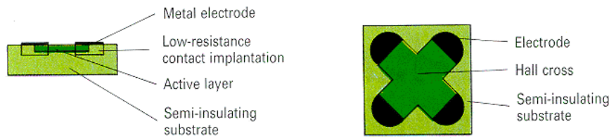
Fig. 2 Structure of GaAs chip (section and plan view) of KSY14 Hall sensor
